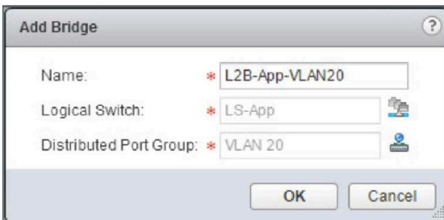
**Figure 2-12** Configuring a Layer 2 Bridge in VMware NSX
