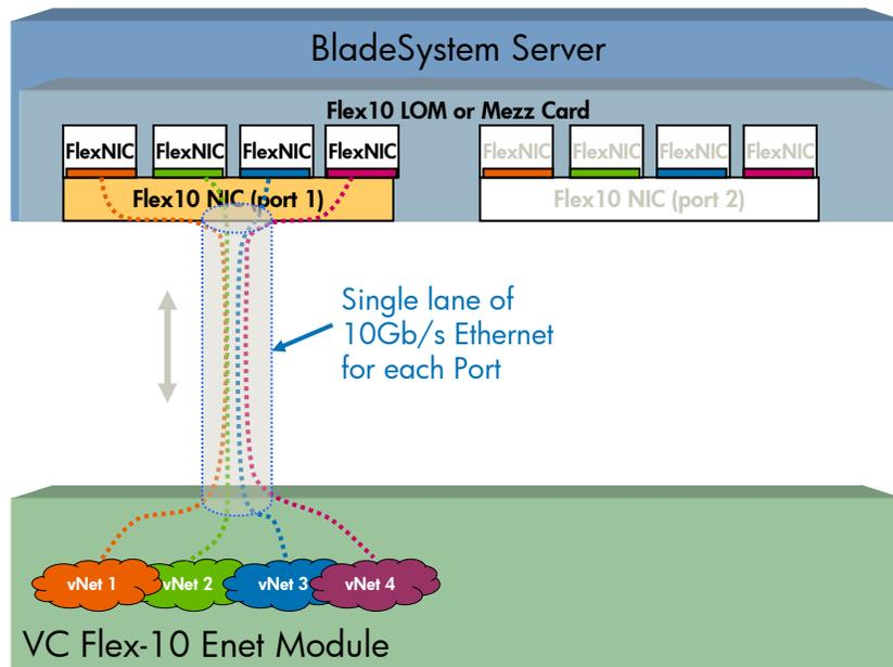
Flex-10 technology complements virtual machine technology by providing a large I/O bandwidth, multiple hardware-virtualized NICs, and the ability to change the bandwidth allocated to each FlexNIC.
