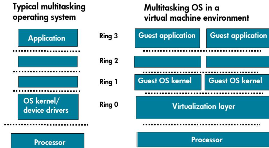
With processor-assisted virtualization, hypervisor software will be able to run in a more privileged ring layer. This will allow guest operating systems to run in their normal ring 0 layer. In addition, AMD-V and Intel VT-x include new instructions that are specific to hypervisors. The combination of these two factors (higher-privilege ring level and new hardware instructions) may provide a more efficient way for hypervisors to virtualize server hardware.
