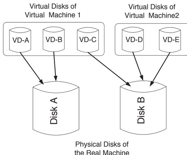
Figure 2: Mapping of Virtual to Physical Disks.
