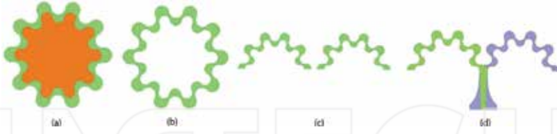
Figure 5. A method to use ASCCC fractal in arms of an antipodal dipole antenna (a) two first-order ASCCC fractal with same n_1 but different R_1 are designed, (b) inner fractal is subtracted from the outer one, (c) the shape is split into two equal halves and (d) each half is employed as an arm in an antipodal dipole antenna [5].
