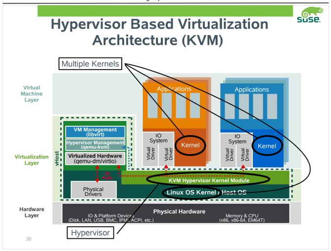
With KVM (or the Kernel Virtual Machine), a kernel module is loaded into the Linux kernel that turns it into a hypervisor. KVM would essentially be a Type I Hypervisor because it is running directly on top of the hardware.
