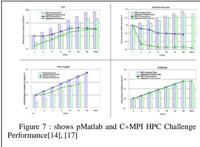
Figure 7 : shows pMatlab and C+MPI HPC Challenge Performance[14], [17]
