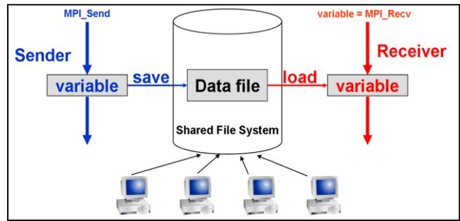
Figure 3: MatlabMPI file I/O based communication[14].
