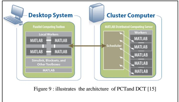
Figure 9 : illustrates the architecture of PCTand DCT [15]
