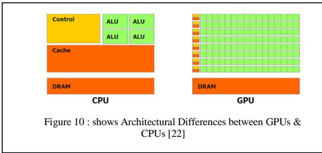
Finally, the architecture of GPUs can be classified as Single Instruction Multiple Data (SIMD).
