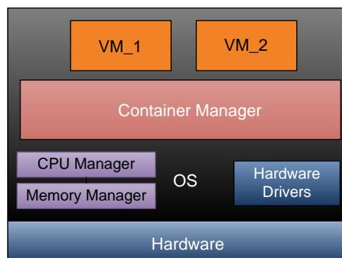
OS virtualization divides a single host OS into containers and uses a container manager for management. It does not use a traditional hypervisor to manage VMs.
