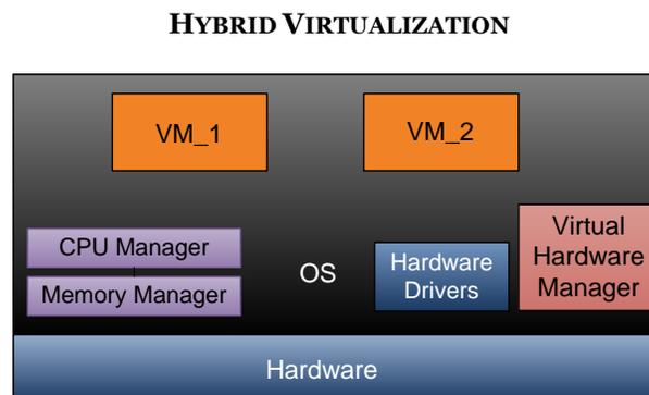
Hybrid virtualization uses a host OS like hosted virtualization, but instead of running a hypervisor on top of the host OS, a Kernel-level virtualization driver is inserted into the host OS kernel. This driver acts as a Virtual Hardware Manager (VHM sometimes called a Virtual Machine Monitor), coordinating hardware access between the VMs and the host OS. Because the VHM accesses hardware directly, especially the CPU, Hybrid virtualization is also called Hardware-Assisted Virtualization.
