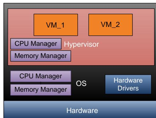
Hosted virtualization approach relies on having an existing operating system (OS) in place. The hypervisor runs on top of the OS, and the virtual machines (VM) are managed by the hypervisor. Note that there is a memory manager and central processing unit (CPU) manager (scheduler) in both the hypervisor and the host OS. This creates a large amount of overhead.
