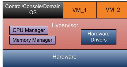
Here the hypervisor sits directly on top of the hardware—hence the term “bare-metal virtualization.” Note that hardware device drivers are part of the hypervisor and that only one CPU/Memory manager is present.
