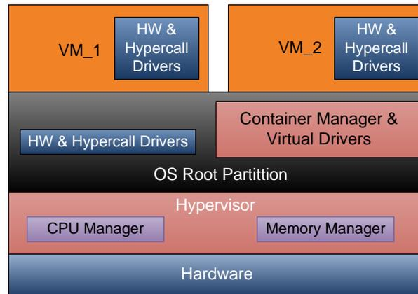
The newly released Microsoft Hyper-V virtualization product employs elements of both the Bare-Metal and Hybrid architectures. Specifically, there are both kernel-level drivers (hybrid) and a hypervisor with VM containers (base-metal). Since this product requires CPU virtualization extensions, we feel this is more a hybrid architecture product than a bare-metal product. However, Microsoft positions Hyper-V as a competitor of VMWare ESX.
