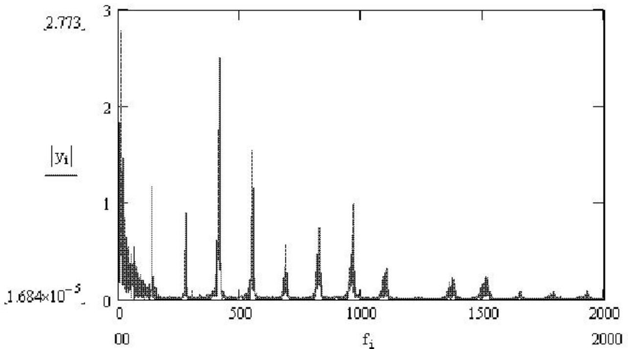
Note that this graph is very “spiky.” In other words, even though the reed’s waveform includes all frequencies, most of the power of the signal is at a few frequencies which arise from the physical properties of the reed.
