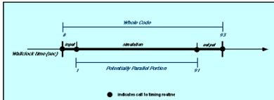
[Figure 8](#). Timing the baseline program to estimate likely parallel performance: whole-code versus potentially parallel timings.
