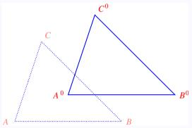
The bold triangle A'B'C' is an exact replica of the dotted triangle ABC, only shifted to the right a little. Having drawn ABC, if we can shift the coordinate system to have the origin at A', then the same code could be used to draw A'B'C' also. This can be done by (re)setting the parameter origin in the code for drawing A'B'C'. Thus the above picture (without the labels, as usual) can be drawn as shown below:
