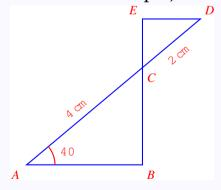
Taking A as (0,0), we can specify C and D by polar coordinates as (4;40) and (6;40). Using the technique just described, B can be specified as (4;40|0,0) and E as (4;40|6;40). Thus this figure (without the labels, of course) can be produced as shown below:
