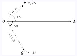
If the distance OP is equal to r and  $\angle AOP$  is equal to  $\theta$ , then r and  $\theta$  are said to be the *polar coordinates* of P and P is labeled  $(r, \theta)$ . Thus in the picture above, P has polar coordinates (2, 45) and Q has polar coordinates (3, -60). Note that Q can also be represented as (3, 300) (and P as (2, 405), for that matter).
