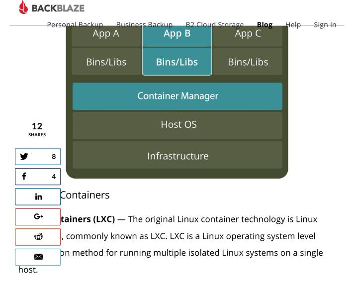
**Docker** — Docker started as a project to build single-application LXC containers, introducing several changes to LXC that make containers more portable and flexible to use. It later morphed into its own container runtime environment. At a high level, Docker is a Linux utility that can efficiently create, ship, and run containers.
