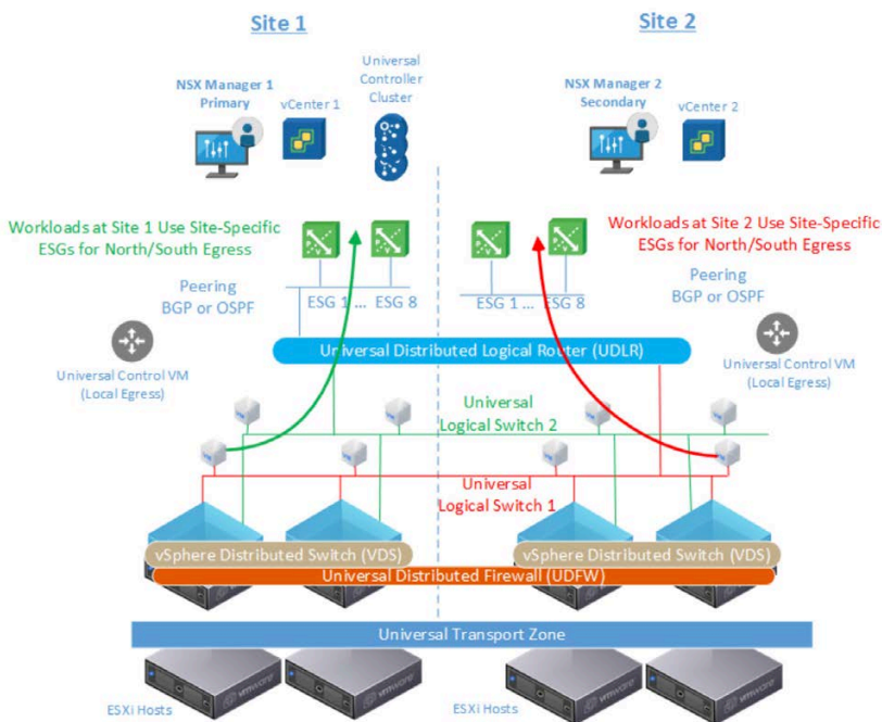
Figure 7.26 Site-specific Active/Active North/South Egress Enabled by Local Egress
