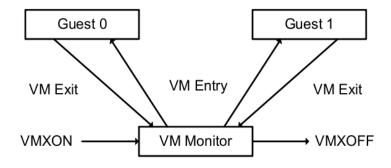
Figure 2: Interaction of a Virtual-Machine Monitor and Guests
