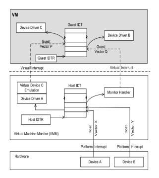
Figure 5: Host External Interrupts and Guest Virtual Interrupts
