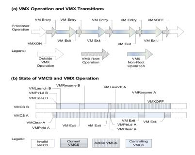
Figure 7: VMX Transitions and States of VMCS in a Logical Processor
