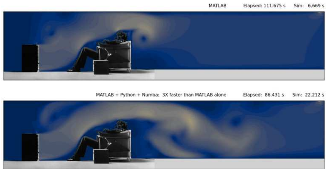
Figure 13.1: Upper panel: air flow computed with MATLAB 2022b using a Navier-Stokes solver by Jamie Johns . Lower panel: air flow computed with MATLAB 2022b calling the same code translated to Python with Numba. It repeats the simulation more than three times in the amount of time it takes the MATLAB-only solver to do this once. Animation on YouTube
