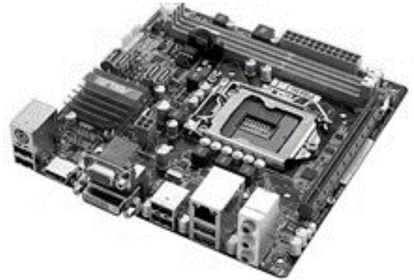
Fig. 2 Tarjeta Micro ATX
