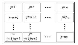
Thus, the plot at location (i,k) is subplot number j = (i-1)m+k. To fill the window with plots you need to call function  $mtlb\_subplot$  a total of p times using fixed values of m and n and varying j according to the position of the plot.
